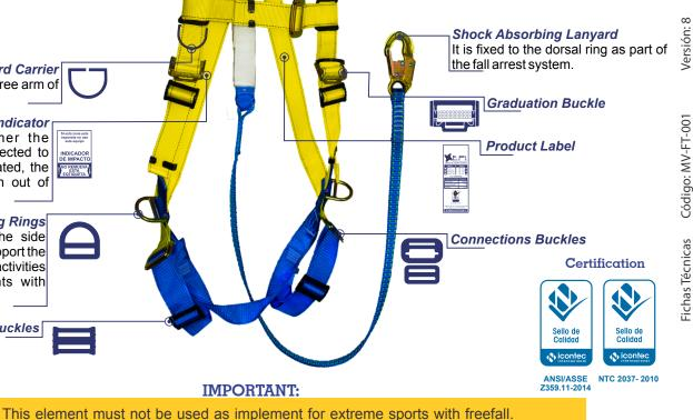
Lanyard: Shock absorbing system lanyard certified under requirements ANSI Z539.13 for falls about 6ft (1,80m), made of 25 mm polyester webbing and safety hook with double safety system and <sup>3</sup>/<sub>4</sub> (21mm) opening. The lanyard length before activation is 1.80m.
